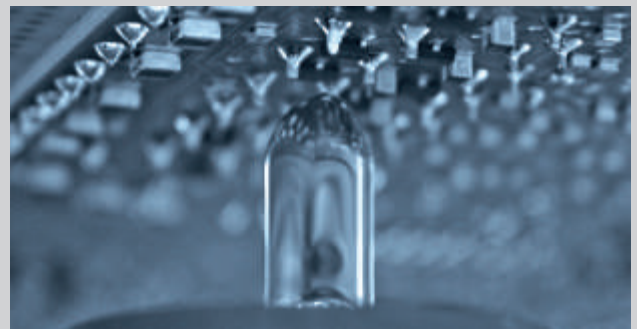
highest flexibility and precision in selective miniwave soldering
