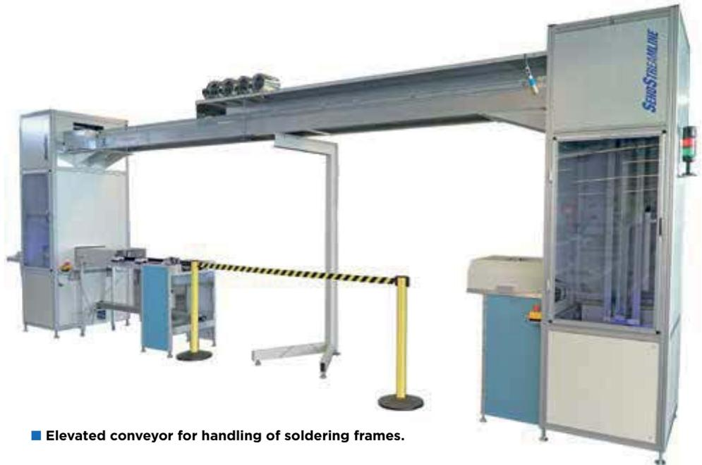
■ Elevated conveyor for handling of soldering frames.
