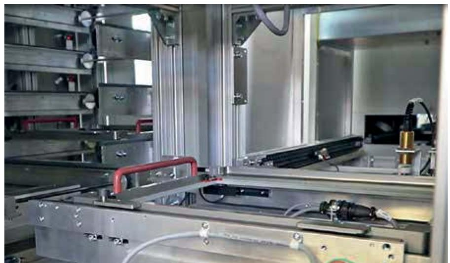
■ Turning station: change of the soldering frames’ travel direction and synchronizing workstations.
