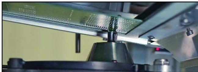
*Soldering process with a 7° angle – perfect peel-off and minimization of potential soldering defects.*
