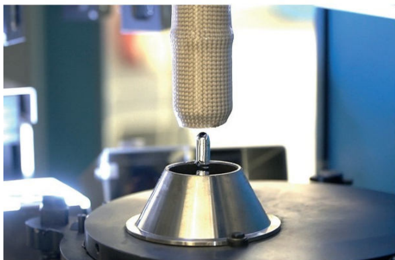
The automatic ultrasonic cleaning for wetted solder nozzles ensures a safe process and increases system availability. Source: SEHO Systems GmbH
