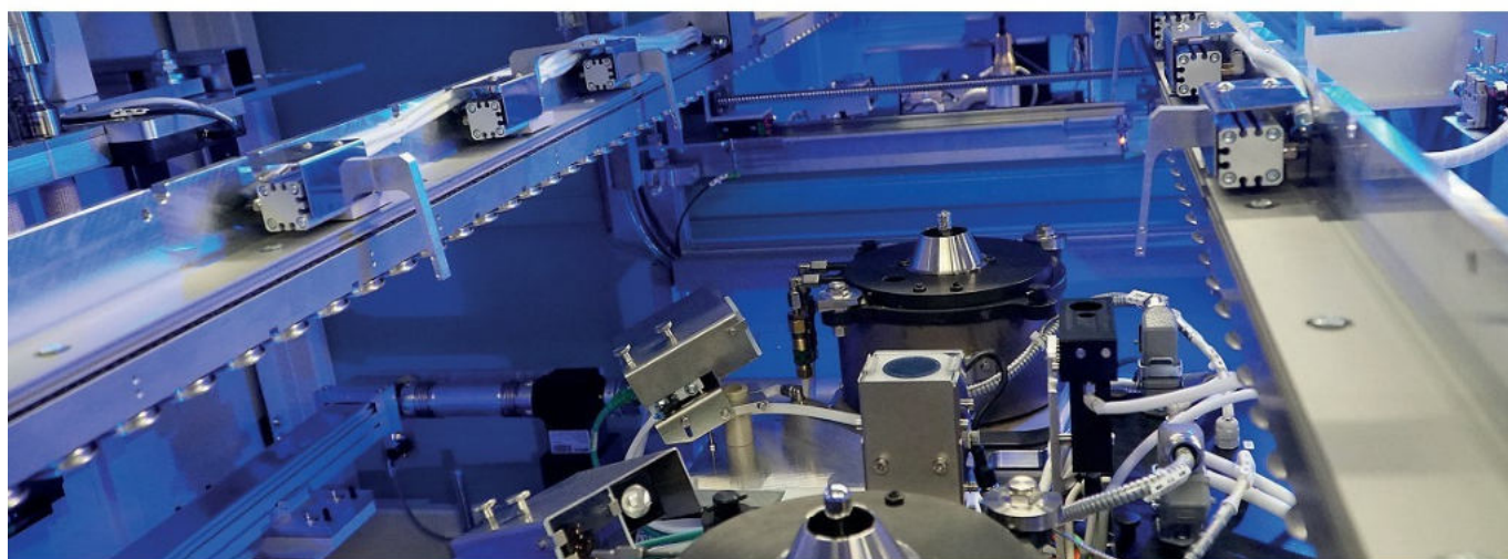
The modular SelectLine can be equipped with more than 15 parallel work stations. At Siemens Amberg, the system is designed for flexible high mix high volume production. Source: SEHO Systems GmbH
