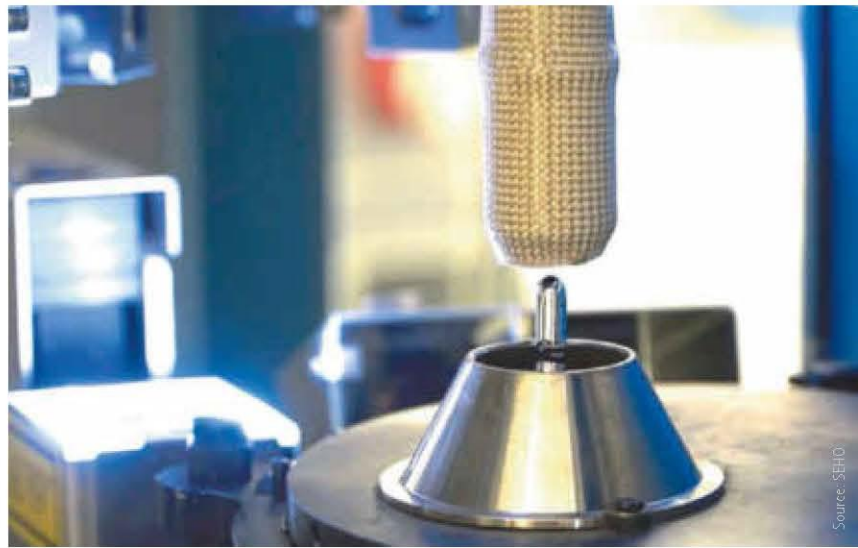
The automatic ultrasonic cleaning system vibrates the liquid solder, cleaning and rewetting the nozzle surface without atmospheric oxygen
